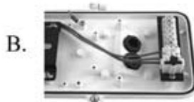
B. Creating an additional 60mm of internal camera space
